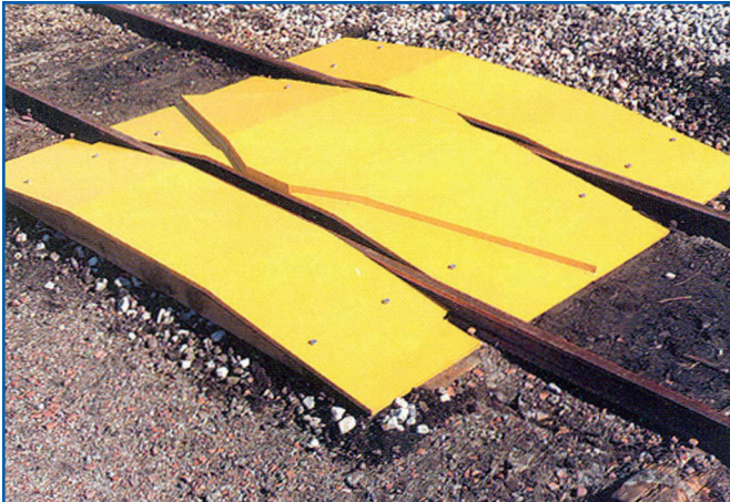
The Nolan Company's PAR-1 Bi-directional Rerailer installed on track.
