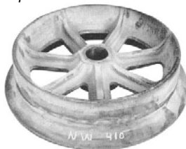
Nolan special ductile alloy wheel after 100.0 hours under 5,000-lb. load shows normal wear.
