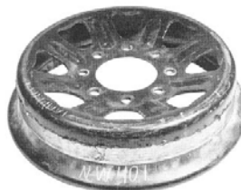
Pressed steel wheel after 31.4 hours under 2,500-lb. load shows EXTENSIVE wear.
